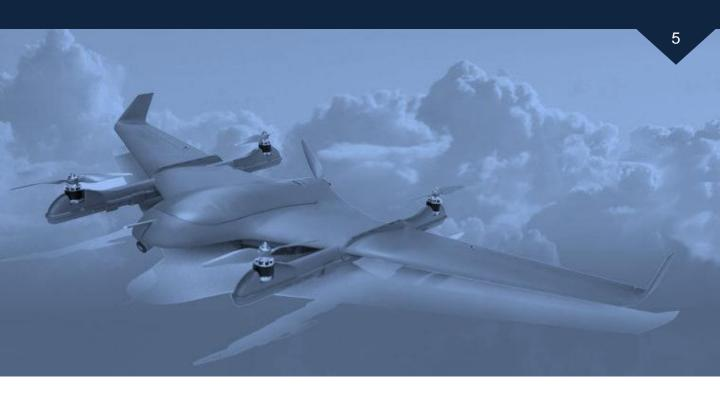
**TRISTAR** is a composite vertical take-off and landing VTOL design UAV and designed and manufacturing by Sparkle Tech profession team, applies fixed wing combined with the quad-rotor complex fixed wing layout, which solves the problem of vertical take-off and landing in a simple and reliable way.
