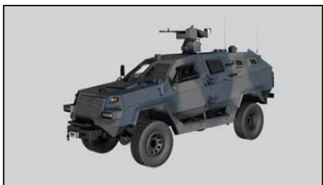
Remote controller weapon station with 12.7x108 mm NSV machinegun
