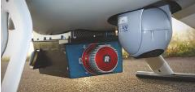
Payload Example with EO/IR and LiDAR
